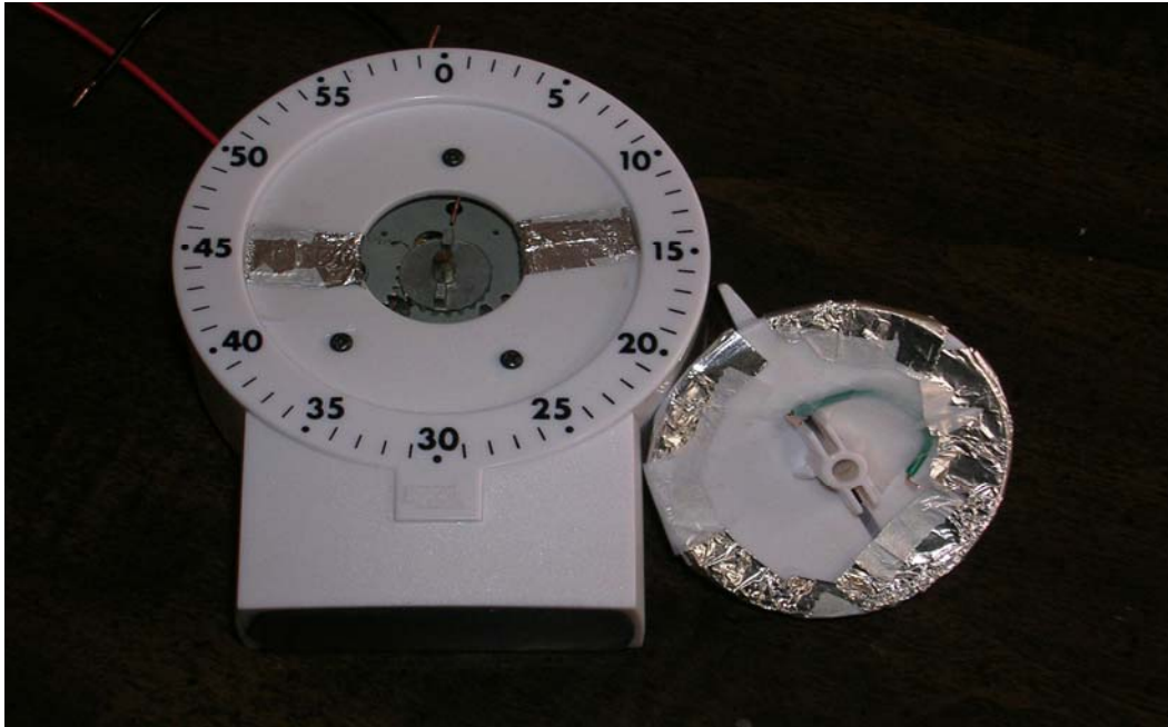
Figure 1: A view of the timer switches
