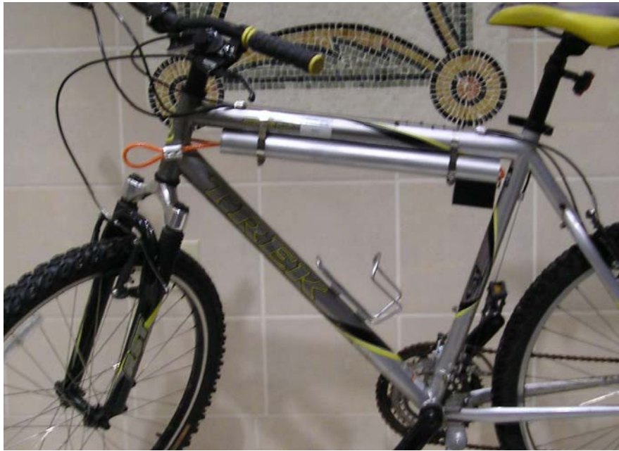
Figure 1: Side View of Cable Housing With Retracted Cable
