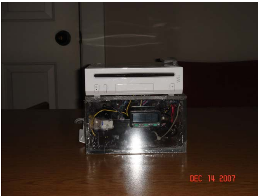
Figure 2: Outside project: Wii on top of the Plexiglas box and temperature controller.
